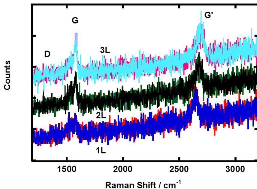
Figure 1. Representative micro-Raman spectra collected from 1L, 2L and 3L graphene regions after the deposition of 10 nm Ni thin film.
